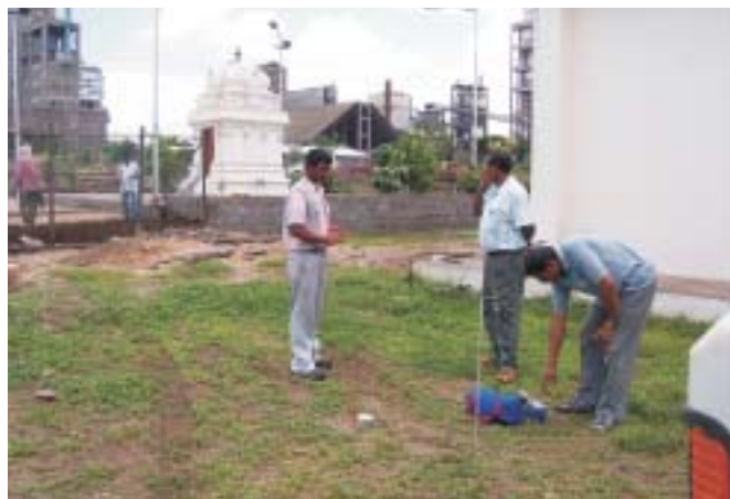
Ground vibration monitoring undertaken by Mining Research Cell, IBM at Parasakti (Jettipalem) limestone mine of M/s Parasakti Cement Industries Ltd., Distt. Guntur, Andhra Pradesh
