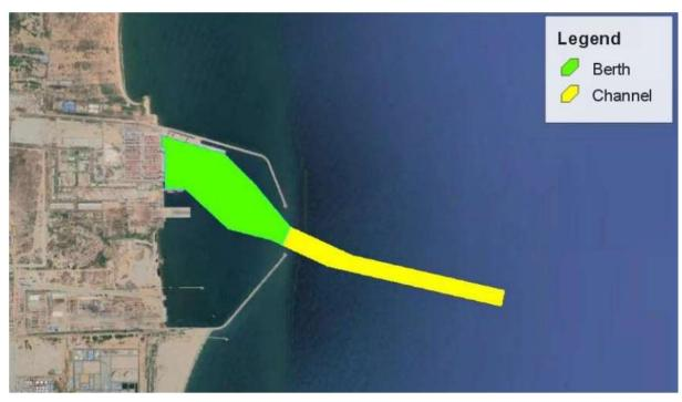
Figure 4-36: Existing dredging layout for kattupalli port
